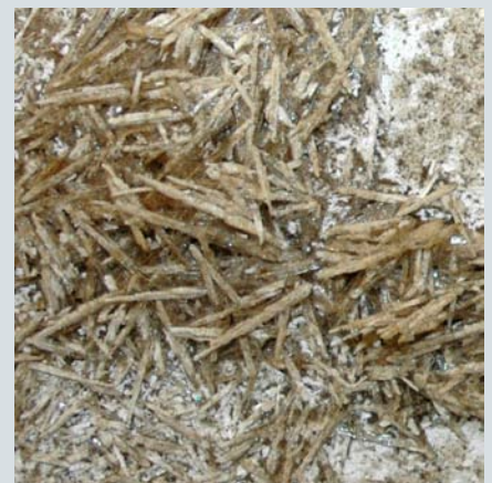
\text{CaSO}_4 crystals in sludge after hydrocyclone and drying
